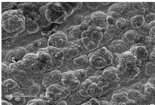
Fig. 6. SEM micrograph of Ni–Co deposit upon annealing at 823 K (alloy 1 prepared from the electrolyte with concentration ratio \text{Ni}^{2+}/\text{Co}^{2+} = 4 at a current density 65 \text{ mA cm}^{-2} ; magnification 2000\times (SE, accelerating voltage 10 \text{ kV} ).
